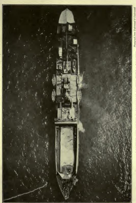
The British use specially equipped ships such as this from which balloons may make ascensions for observing the enemy's positions. The ascensions are made from the deck between the bridge and bow A BRITISH SHIP AT THE DARDANELLES AS SEEN FROM A BALLOON
